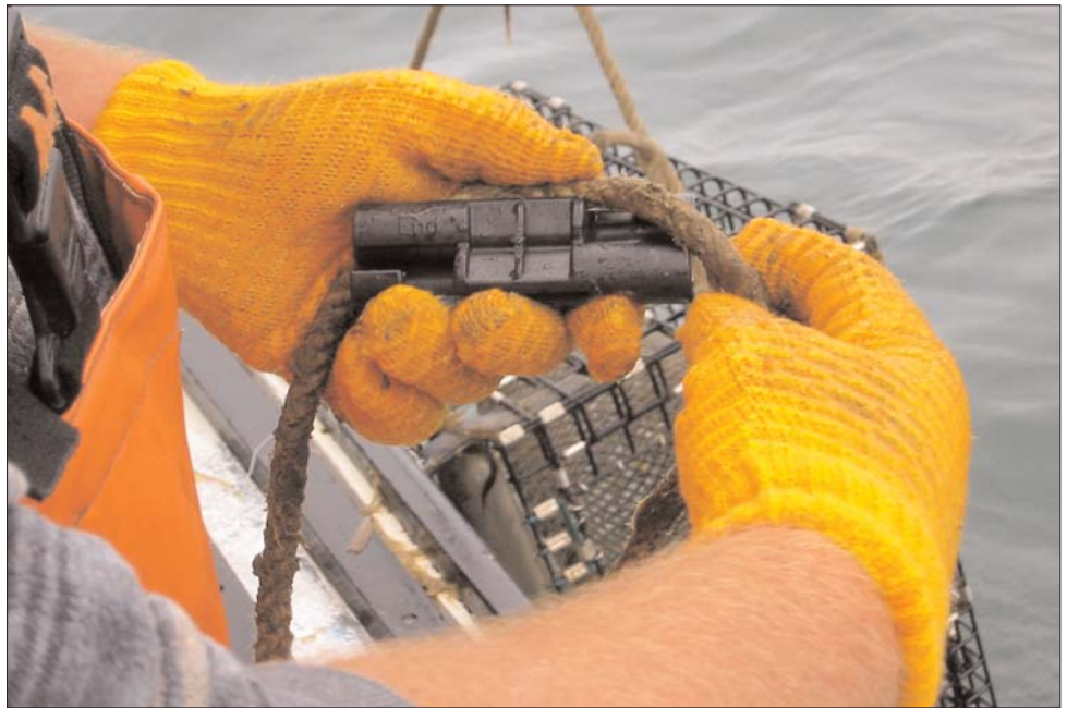
The device attaches just below a buoy. The bitter-end of the line sits 12-inches away from the cylinders to prevent accidental slipping.
