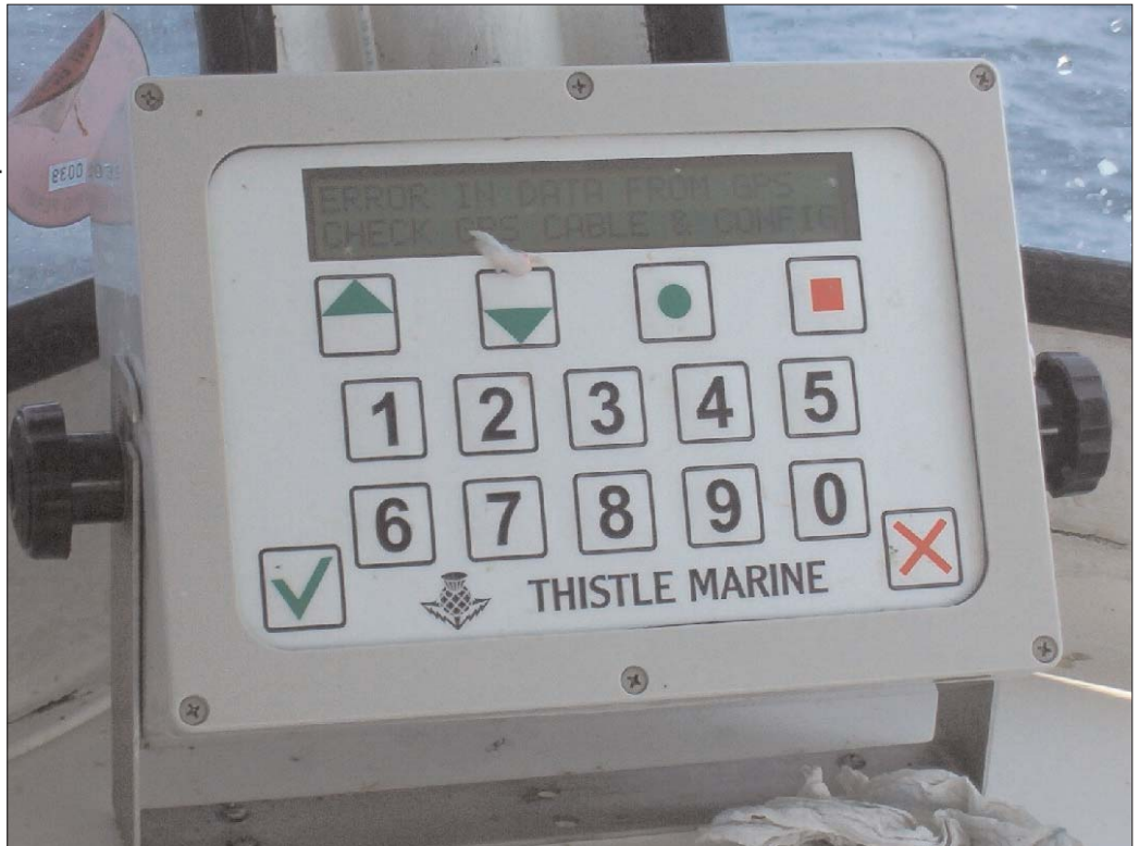
Old Standby: The Thistle Marine HMS-110 data collection device. (Image courtesy of NOAA)
