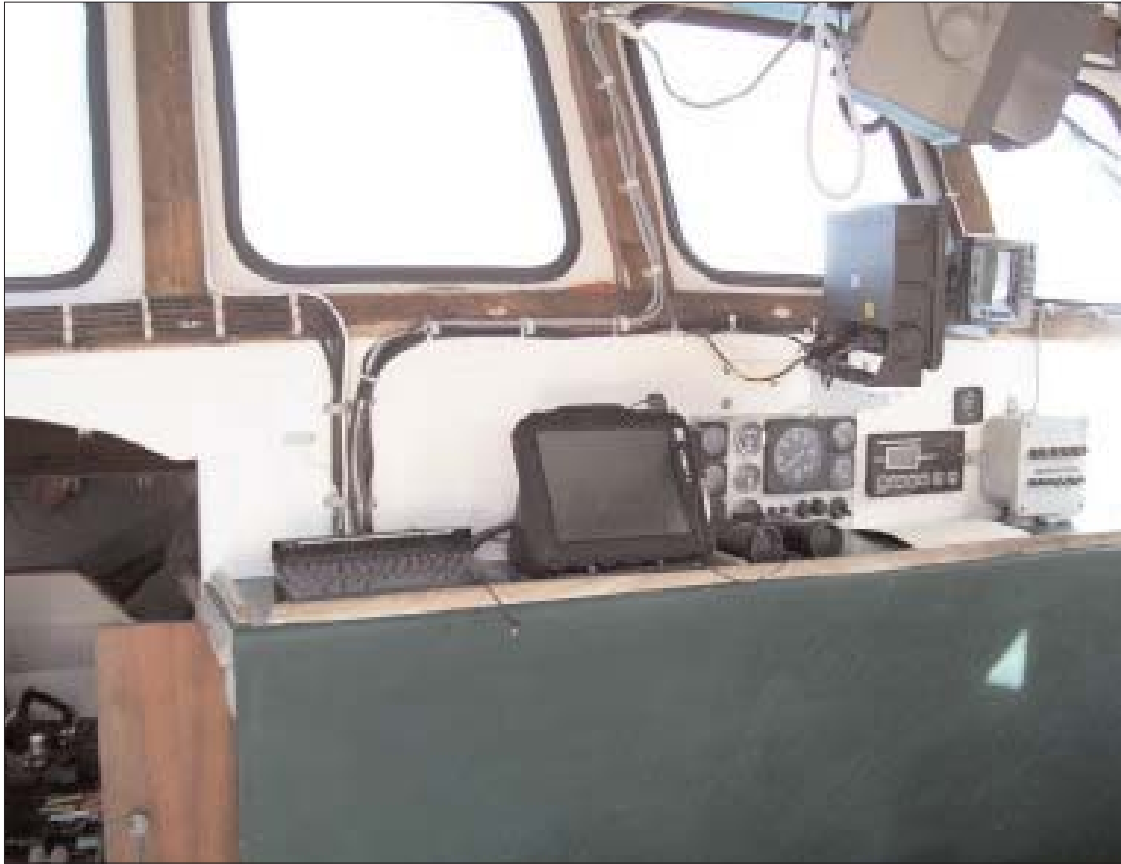
The Walkabout Hammerhead, an example of a tablet PC. (Image courtesy of NOAA)
