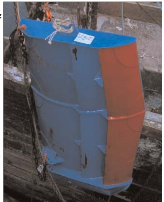
Image courtesy Pingguo He: The trawl door.
