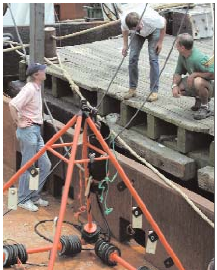
(Images courtesy of SMAST) Top: A GIS-based image of the sample area shows the project's enormous scope, from Georges Bank to Virginia. Each dot represents an individual sample station. Bottom: Dr. Kevin Stokesbury stands with the "sampling pyramid." The device supports video cameras at a fixed distance from the base.
