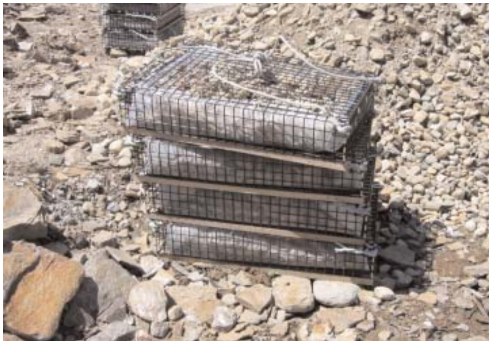
10-gauge vinyl-coated wire with 2-inch mesh. Each measures 24 x 33 inches in the floor and 6 inches deep. For strength, the upper edge was bent inward to make lip to clasp the wire cover. Chris Manning photo.
