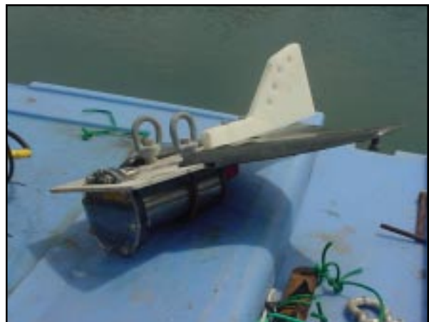
IT'S A BIRD. . . IT'S A PLANE. . . Actually, it's just another of Bill Lee's underwater cameras with a frame designed to be towed near the boat's bow
