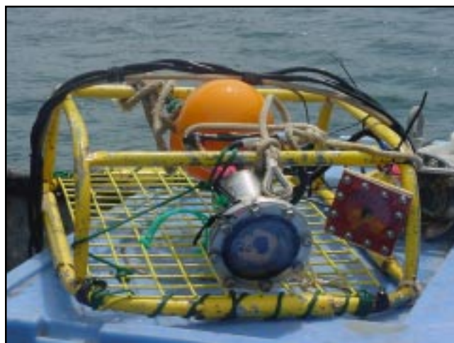
BUILT FOR ABUSE — Two of Bill Lee's underwater cameras are mounted in this homemade frame. The camera on the right (with the red flange) shoots black and white images; the other camera shoots in color. Lee says he designs the cameras and their frames to handle the rigors of being used on a commercial fishing vessel.
